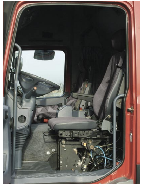
The prototype of the active seat suspension, integrated into a driver's cab.
