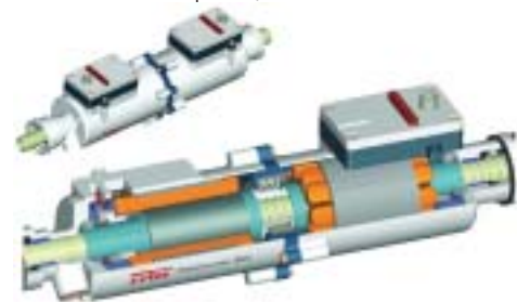
▲ Steer-by-wire front axle actuator.
