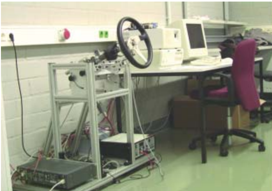
▼ CIL test bench with force feedback actuator.
